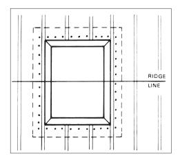
C 6. Fasten roof panel through curb flanges to support steel using suitable fasteners compatible with roof system. A minimum of four fasteners per side spaced on 3" centers or less as roof system permits. Fasteners should withstand a minimum pullout force of 150# each.
